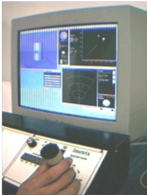
**Figure 2.** Simulated ROV operator station
