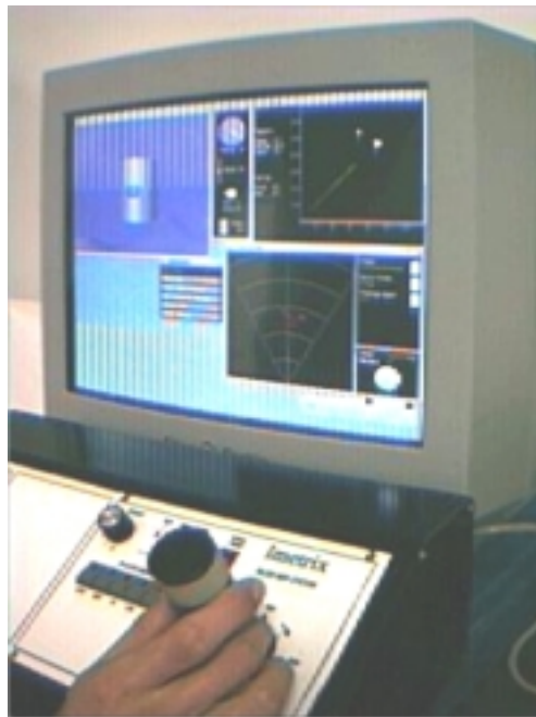
Figure 2. Simulated ROV operator station
