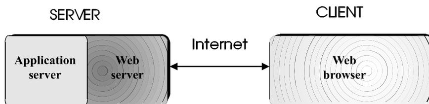
Fig. 1. Centralized architecture
