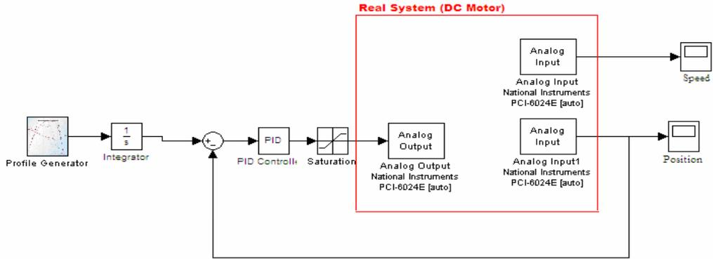
(b). closed loop with PID controller.
