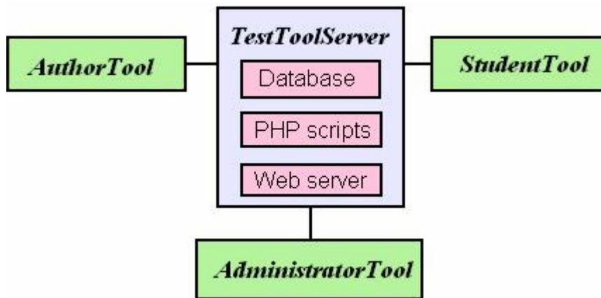
FIGURE 1: TestTool structure
