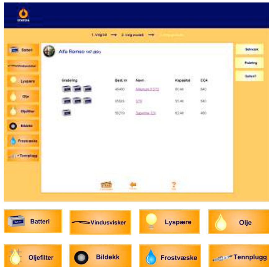
Figure 4: Second prototype (laptop interface) created by the researchers based on the feedback from the first prototype. The emphasis of this prototype was to improve the user interface of product information and ease navigation. The bottom view shows a close-up of the navigation icons.
