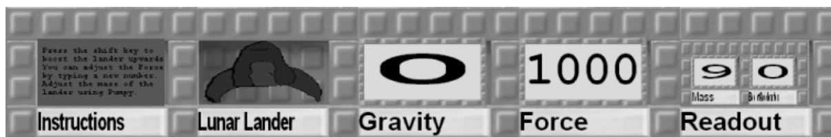
Fig 5. Booster tool provided to students. The lunar lander is taken out of the box and placed on the floor. 'Gravity' and the 'Force' can be set simply by typing numbers on the controls. When the 'shift' key is pressed, the 'Boost acceleration' is determined. The 'Gravity' setting simply accelerates the lander by that value. The mass of the lander is determined by its size, which can be directly controlled using the built-in ToonTalk bicycle pump tool.
