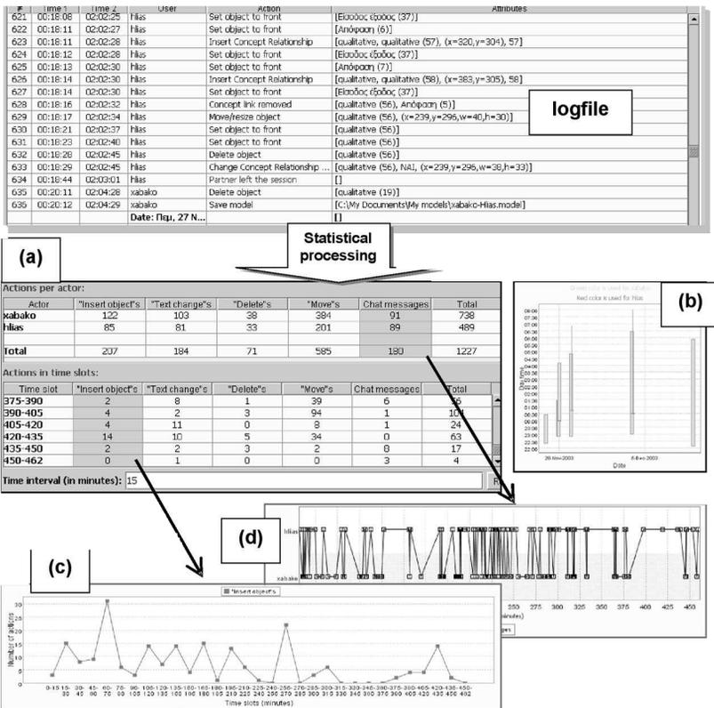
**Figure 1.** Synergo analysis tools: The log file (top of the picture) is processed for producing statistical indicators across various dimensions (type of event, time slot, actor), shown in (a). Also, the group sessions over time are shown in (b), while in (c) and (d) the statistical indicators are plotted vs. time
