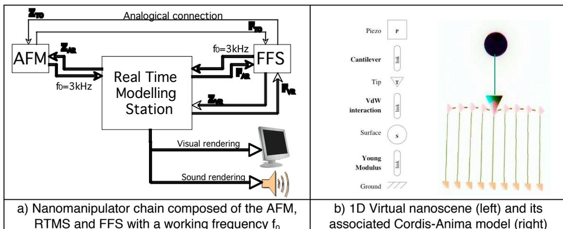
**Fig. 2. Multisensory platform**
